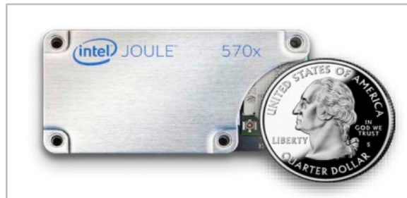
Intel Joule 570X (1.7 GHz, Quad-Core, 4 GB RAM, 16 GB storage)
