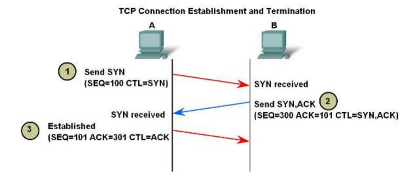
A sends SYN request to B B sends ACK response and SYN request to A A sends ACK response to B
