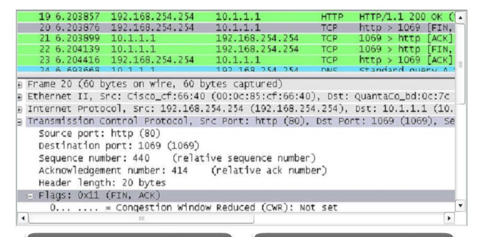
A protocol analyzer shows details of frame 20, TCP FIN request.
