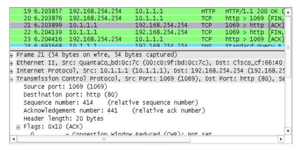
A protocol analyzer shows details of frame 21, TCP ACK response.
