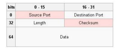
\* Source port: This field identifies the sending port when meaningful and should be assumed to be the port to reply to if needed. If not used, then it should be zero.
