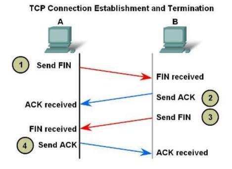
A sends FIN request to B B sends ACK response to A B sends FIN request to A A sends ACK response to B
